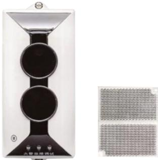
**AT-FA-CBD109** Conventional Reflective Beam Detector is a non-addressable smoke detector with infrared optical beam, with excellent built-in microprocessor, the detector can carry out system adjustment, drift compensation of ambient data, and judgement of fire and fault through fixed algorithm, indicate states through LEDs, provide signals by output relays.
