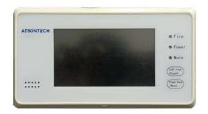
AT-FA-RP2060 Fire Repeater is an intelligent device, and it is designed using a single chip to display position, number and messages of alarming detectors and to send audible and visual alarm signals as well. It is connected with fire alarm control panels, through fire loops to display and process data.
