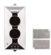
AT-FA-CBD109 Conventional Reflective Beam Detector is a non-addressable smoke detector with infrared optical beam, with excellent built-in microprocessor, the detector can carry out system adjustment, drift compensation of ambient data, and judgement of fire and fault through fixed algorithm, indicate states through LEDs, provide signals by output relays.
