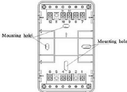
The base of sounder is suitable to be installed onto European style backbox. There are two terminals with marks on the base D1 & D2: 24VDC power supply, non-polarized.
